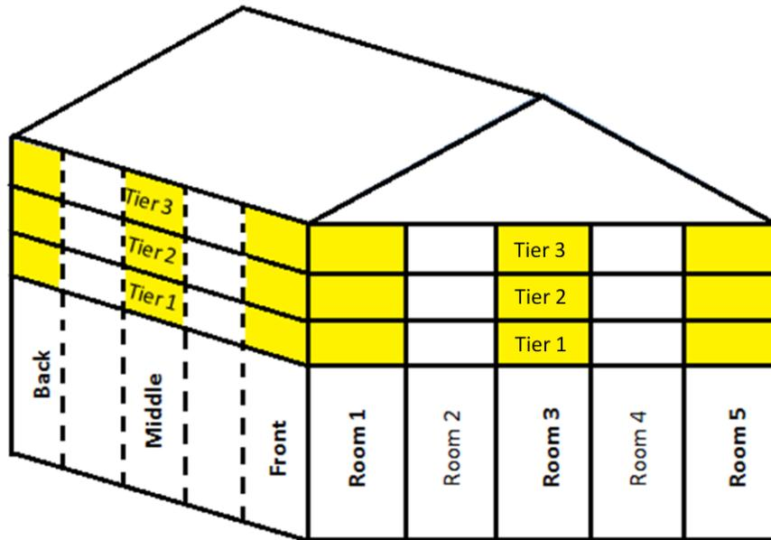
Figure 1.2 Diagram of long-tier orientation barn demonstrating the 3-Dimensional area that was studied.
